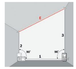
**Trapezium function** for measuring roof slopes.
